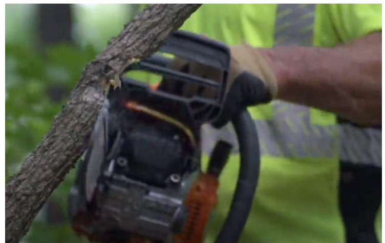
Figure 13. Shave cuts to release tension. A series of shave cuts on the compression side at the point of maximum tension also will safely release a spring pole.
