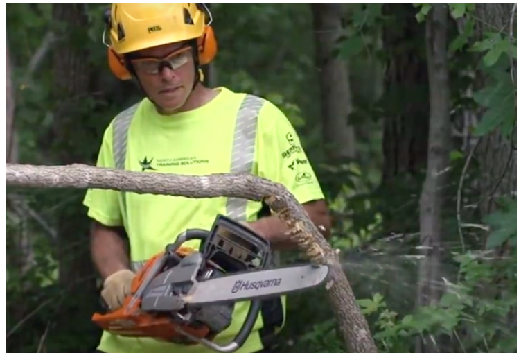
Figure 12. Making an accordion cut. Use a series of small cuts on the compression side at the point of maximum tension to release a spring pole.
