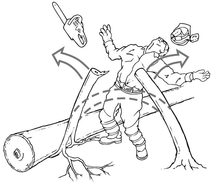
Figure 10. Spring pole can happen when a tree or branch is under great tension as the chainsaw operator cuts into the wood.
