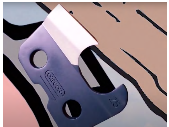
Figure 3. Kickback caused by the saw biting off more than it can chew. When the tooth is in the kickback zone, the depth gauge is lower than it should be in relation to the tooth. The saw cuts a relatively large piece of wood and the chain slows or stops. The force that was driving the chain flings the bar at the operator.
