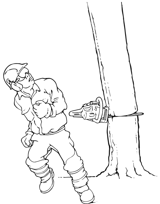
Figure 8. Setback occurs when the tree sets back during the bore cut or back cut, pinching the chainsaw.
